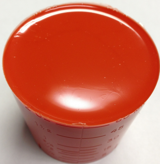
Close-up of cured Matrix™ Urethane Ball Plug. Virtually no air bubbles!
